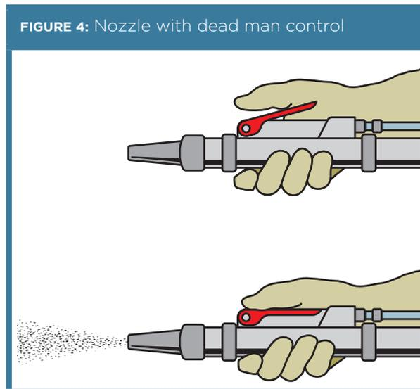
Using a blast machine without a dead man control (under the direct control of the operator) is dangerous and may result in serious injury or death.
