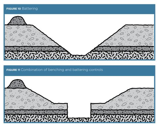
Benching and battering of excavation walls can minimise the risk of soil or rock slipping onto the excavation. Control measures should be designed by a competent person (for example geotechnical engineer) and be relative to the soil type, the moisture content of the soil, the planned height of the excavated face and any surcharge loads acting on the excavated face.
