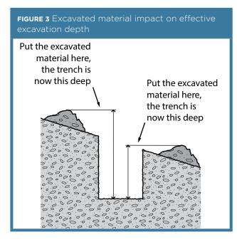
Care should be taken to ensure that material placed on the high side of the excavation does not increase the risk of ground collapse, or flooding by ponding or holding back runoff water. Excavated material should be placed so that it channels rainwater and other run-off water away from the excavation.
