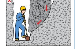
(b) Shear plane failure along the seepage (slippage) plane.
