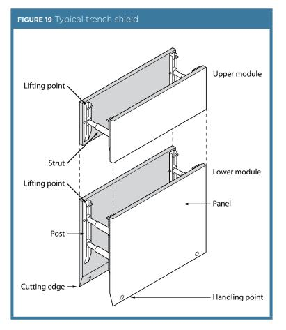
Shields and boxes used in trenches are often referred to as trench shields or trench boxes, and are designed and constructed to withstand the earth pressures of particular trench depths and ground types. They incorporate specific lifting points for installation and removal.
