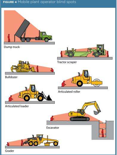
FIGURE 4 Mobile plant operator blind spots
