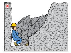
(d) Worker badly injured and probably smothered after being crushed against the opposite wall by the collapsing ground. The weight of a wedge of sand over a one metre length of trench two metres deep is about three tonnes.
