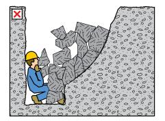
(c) Worker trapped and crushed against the trench wall by the quick collapse.
