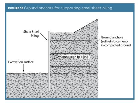
Removal of the soil between the retaining wall and the active soil limit line may cause sheet piling to bend. This bending will release the load in the stressing cable, and render the ground anchor useless and dangerous to workers in the excavation area.
