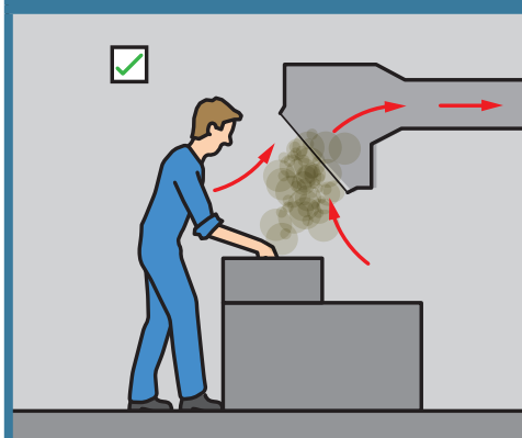
DIAGRAM 4: Good design carries away contaminants from the operator's breathing zone
